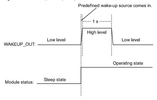
Figure 12-2 WAKEUP\_IN input sequence
